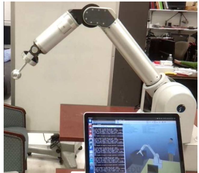
Fig. 4. Screen capture of video taken during experiment. The BMM, running in the laptop (left window), controls in real time both the real WAM arm, via LAN network, and the V-REP virtual WAM arm, running in the same laptop (right window).
